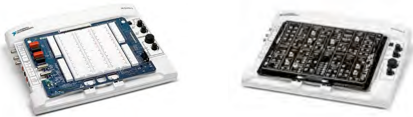
Figure 1. ELVIS for EGR 213 online class (left) and DATEx for WCM 600 onsite class (right).
